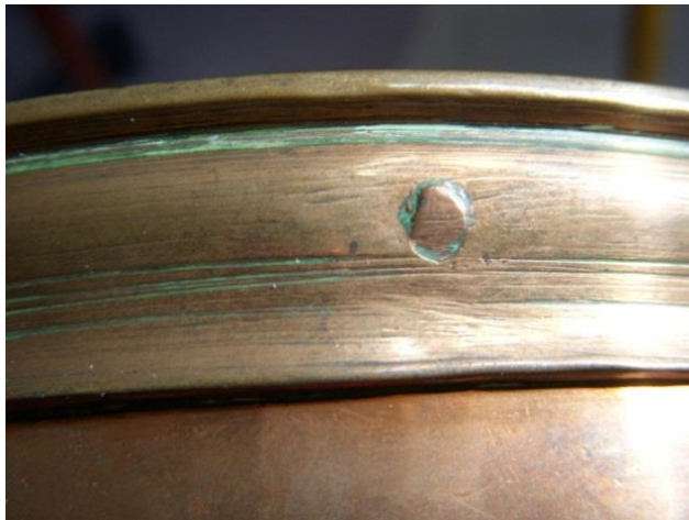
Rim of the 1826 Midland Quart showing the peg in the rim and the mark of the lathe turning that shaped the rim.
