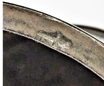
Verification Marks stamped on the Rim Left – Crown over GR III Right – London Guildhall Dagger
