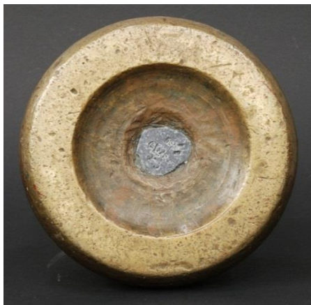
Base of the seven pound St. John's weight showing the lead plug in base
